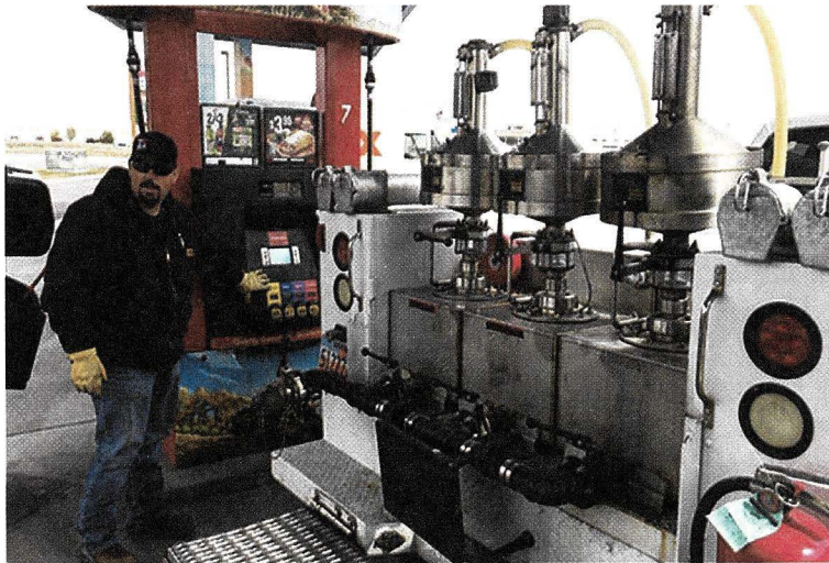
Weights and Measures Inspector, Jeff Jolly prepares to test the accuracy of gasoline pumps at one of the state's more modern gas stations. The division inspected 18,260 gasoline pumps in 2013 to protect both consumer and business interests.
